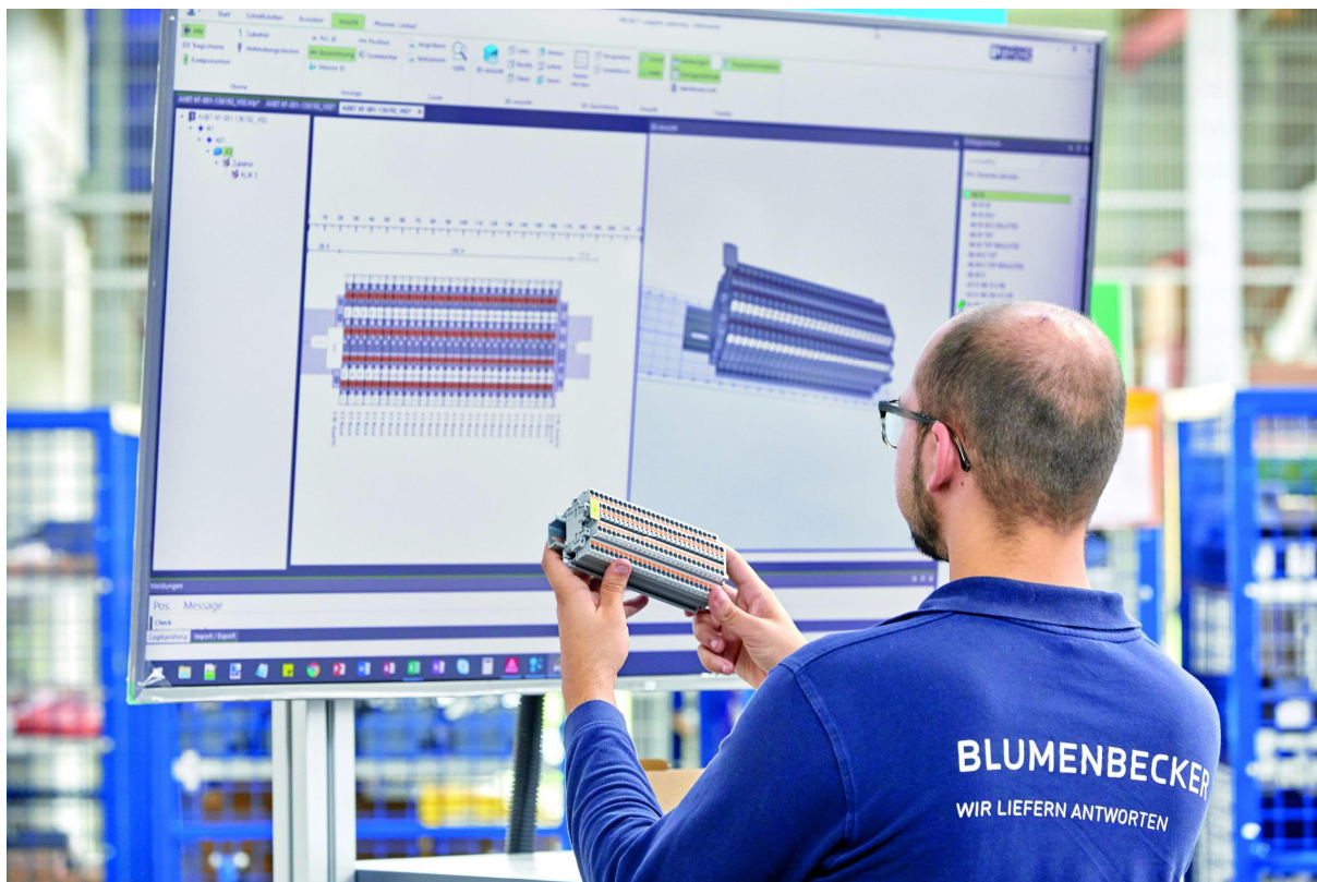
From digital to the real world: The freshly assembled DIN rail is compared to the digital image in the Project complete planning software
